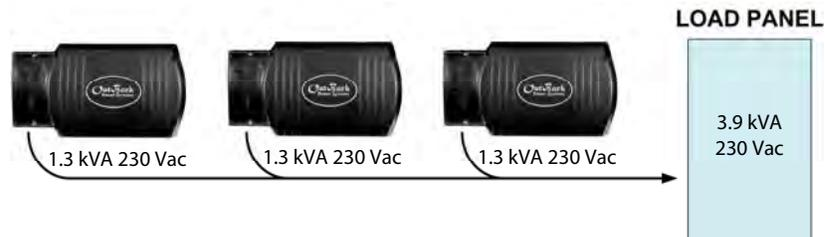
**Figure 7 Example of Parallel Stacking Arrangement (Three Inverters)**
